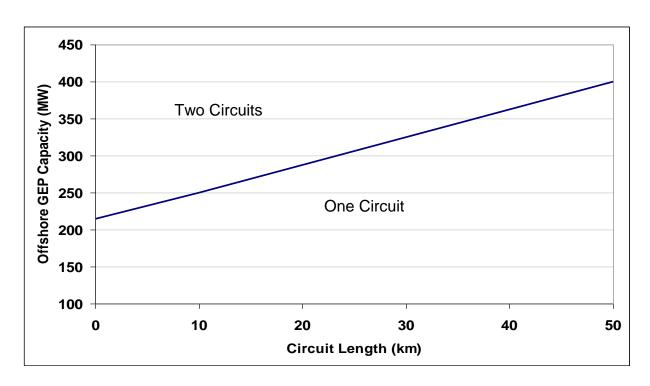
Figure 7.1 Justification for a Minimum of One Circuit or a Minimum of Two Circuits for 132kV AC Overhead Lines
