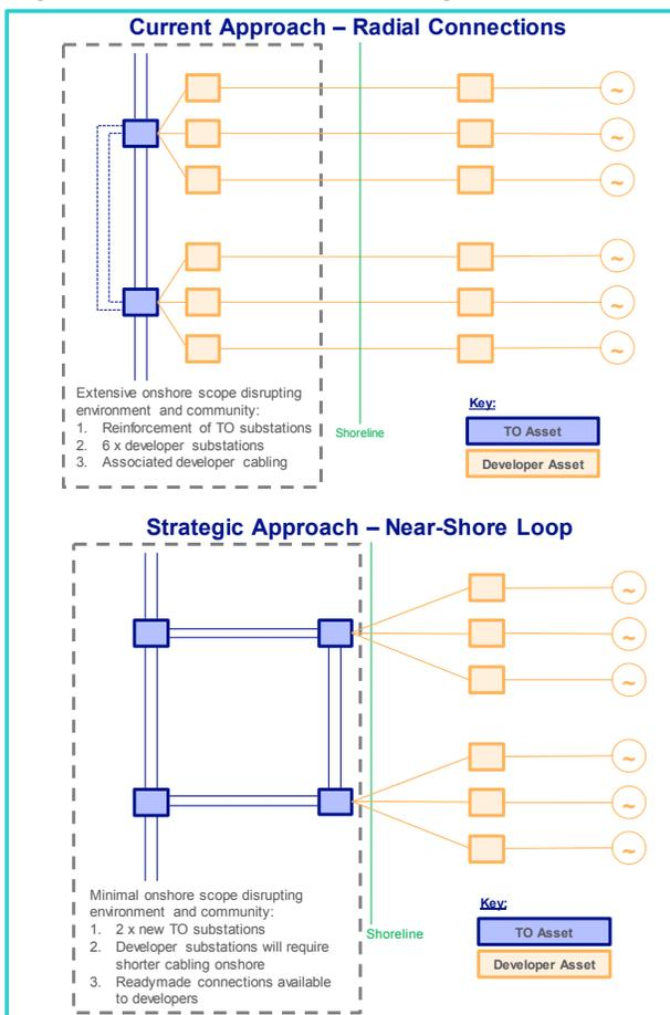
Figure 7.19 contrasts the current radial approach with a coordinated one that would require less onshore construction, minimising cost and disruption. In current costs, we anticipate that this solution would cost between £3bn and £5bn and deliver considerable net benefits for consumers.
