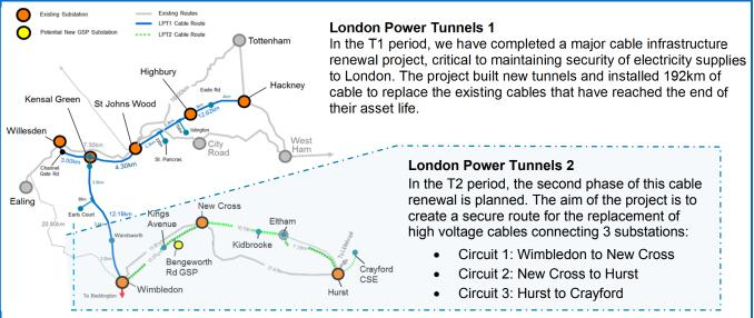
The existing LPT2 cable routes form the sole transmission supply to the New Cross and Hurst grid supply points (GSPs) and provide system interconnection between East and West London.
