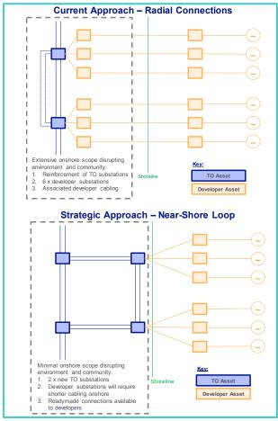
Figure 7.19 Offshore wind topologies
