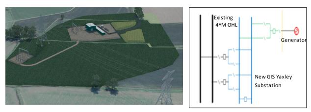
Figure 13: Progress Power Connection and SLD
