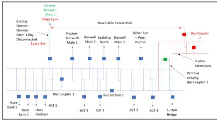
Figure 11: King's Lynn B Connection Layout at Walpole 400kV Substation
