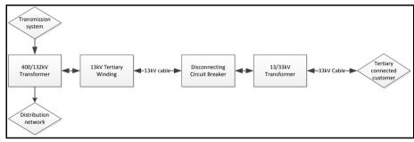
Figure 8: Typical Arrangement for Tertiary Connected Generation
