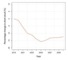
A declining SCL has operability implications related to protection, voltage and stability. The impact of low SCL on the function and performance of protection and control systems is one of the most direct impacts of this trend.
