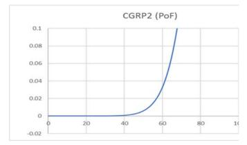
Figure 4: Probability of Failure vs Asset Equivalent Age for cable family type
