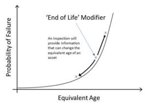
Figure11 illustrates the principle of the End of Life Modifier. The rise in monetised risk is governed by an asset's probability of failure plot, the magnitude of the risk at any given point in time is a function of the probability of failure (variable) and the probability of an event with a monetised consequence (fixed).
