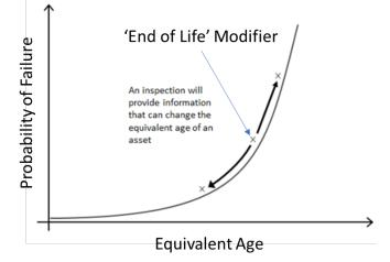
Chart depicting the principle of the End of Life Modifier. The rise in monetised risk is governed by an asset's probability of failure plot, the magnitude of the risk at any given point in time is a function of the probability of failure (variable) and the probability of an event with a monetised consequence (fixed).
