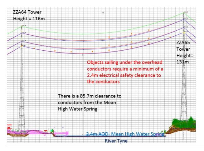
Figure 2: Tyne Crossing- Max clearance to the conductor is 85.7m when the circuits are energised
