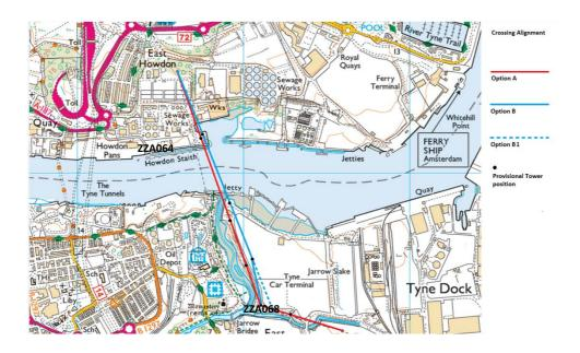
Figure 4: Initial view on OHL diversion. Option A- Red Route is the preferred route
