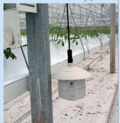
(pictured) that can now be integrated into its all electronic measuring boxes. The cost of maintenance and calibration is said to be a fraction of the cost of more traditional systems that use sampling tubes and pumps.
