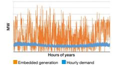
Finally, we investigated if installing batteries, like those used in South Australia, could be an option to allow a region to become selfsufficient. To meet the observed maximum shortfall of 3GW would require the installation of 24 130MWh batteries.
