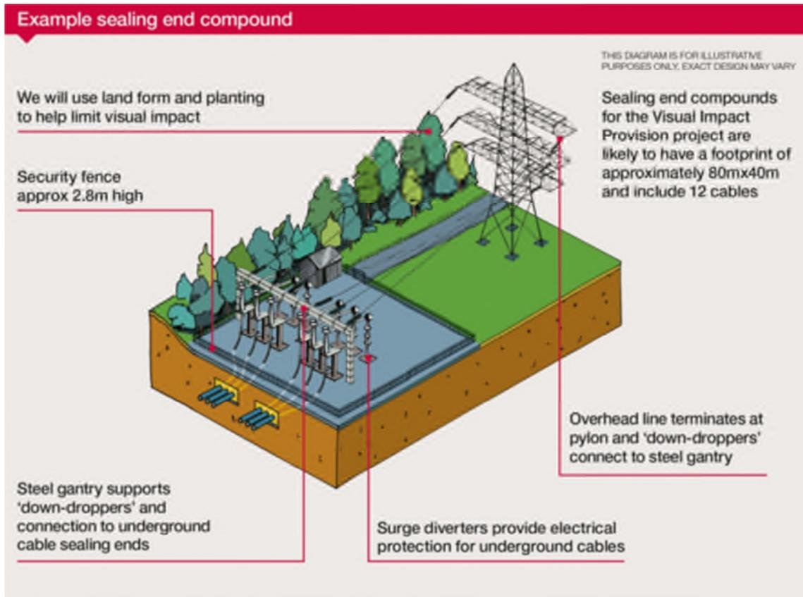
**Figure 5.6 An operational sealing end compound**
